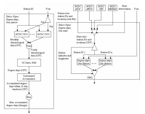
Figure 1: Schematic diagram illustrating how the developers combined different web-based data and analytical services to produce the application.
